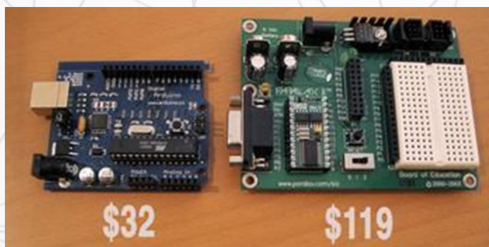
Figura 2 – Arduino vs BASIC stamp (Todbot, 2006)
